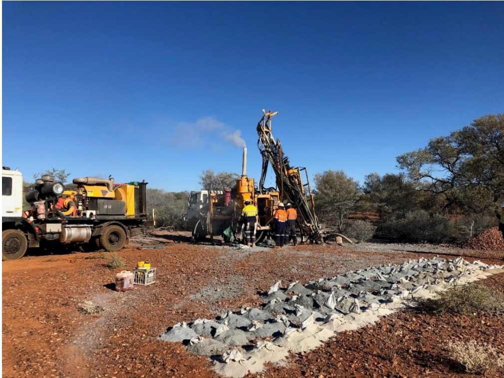
Figure 1: Impact Drilling air core rig set up and drilling the first hole at Green Rocks from Phase 1 of the 5000m air core program.
