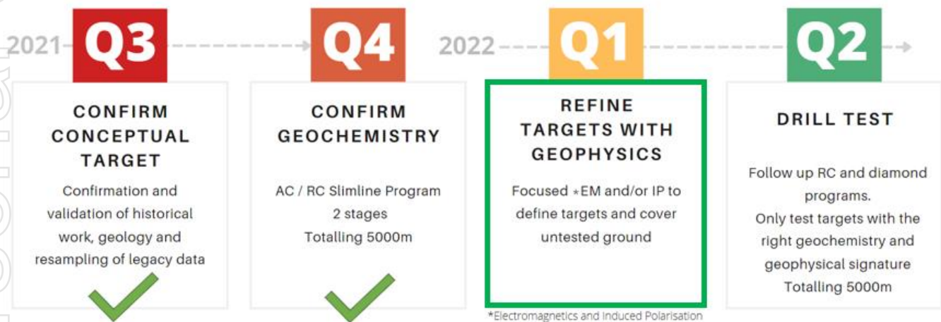
Figure 5: Staged exploration strategy, currently confirming geochemistry through AC Program and refining with geophysics.
