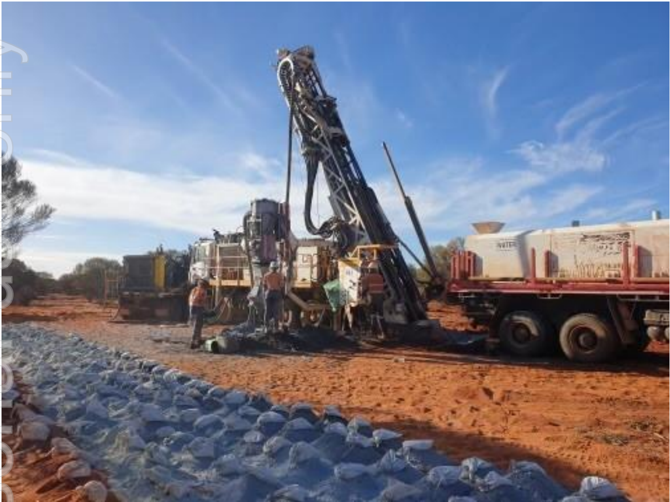
Figure 1. Picture of RC rig at Target B drilling first hole.
