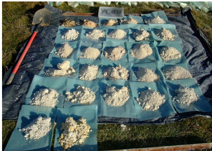
Figure 1. Example of the kaolin intercepts at Yendon from Hole YAC053.
