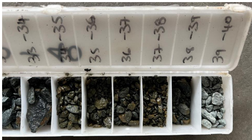
Figure 1. 4m of visible chalcopyrite from 34m to 39m in GRR005.
