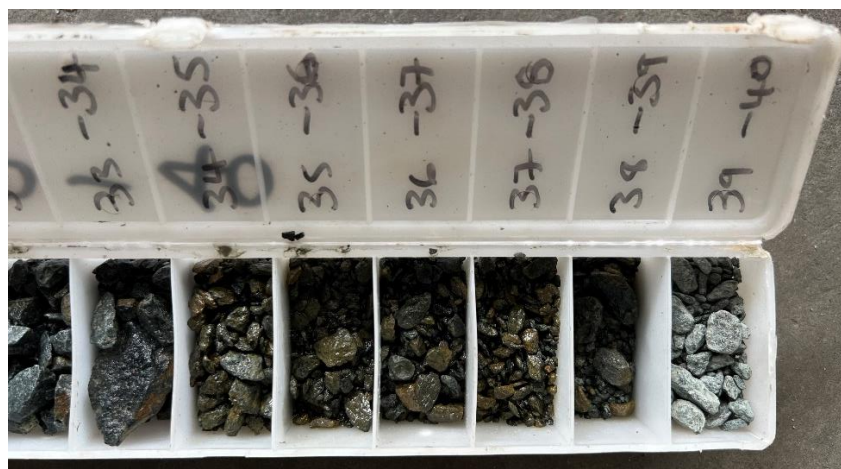
Figure 2. 4m of visible chalcopyrite from 34m to 39m in GRR005.
