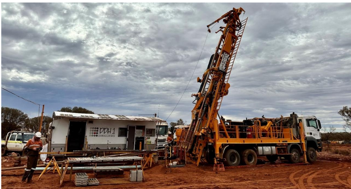
Figure 1: Convertible diamond/RC rig in the final stages of setup to drill 2 holes at Earraheedy.
