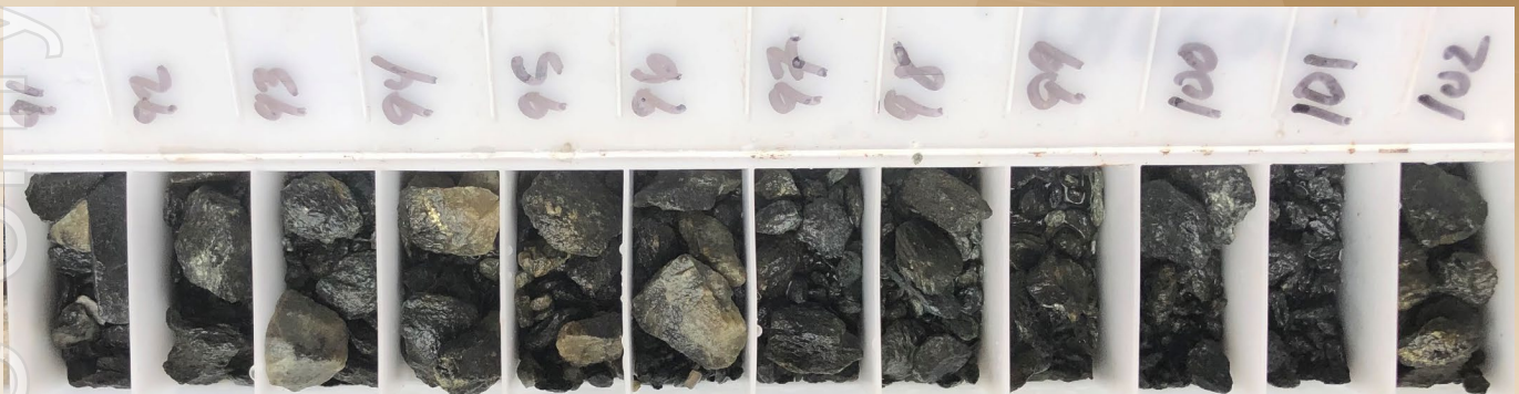
Figure 2: RC chips from CHRC002 which intersected 11m @ 1.25% Cu
