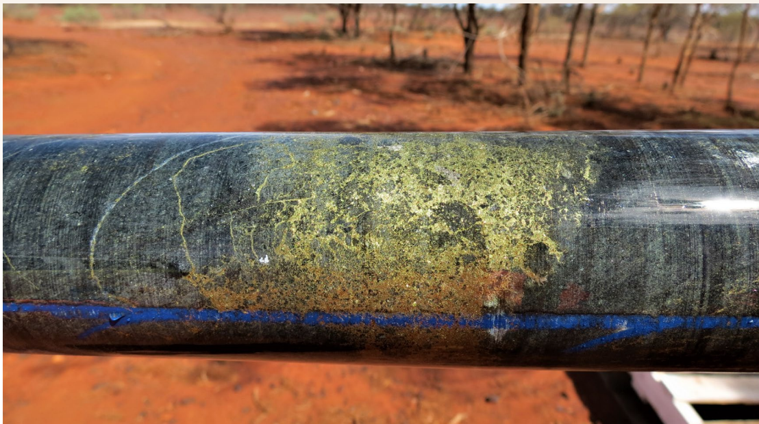
Figure 1: CHD05B-WA from 899.1m- band of semi-massive chalcopyrite with blebs of pyrrhotite
