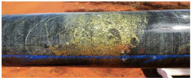
Figure 2: CHD005B-W1 from 899.1m – band of semi-massive chalcopyrite with blebs of pyrrhotite.
