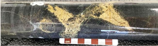
Figure 1: CHD005B-W1 from 827.8 – chalcopyrite in an offset vein.
